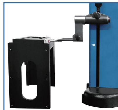
Maximum/Minimum/Difference Value Measurement
